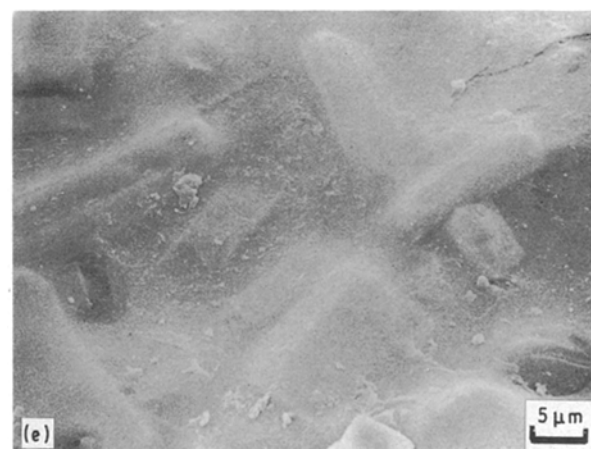
Figure 8 Micrographs of oxidized specimens in an air flow of 0.51\text{min}^{-1} for 54 h (a) Original specimen, (b) 1100^\circ\text{C} , (c) 1200^\circ\text{C} , (d) 1300^\circ\text{C} , (e) 1400^\circ\text{C} .
